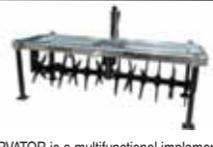
The AERVATOR is a multifunctional implement that relieves compaction, aerates, cultivates and renovates all growing conditions. The AERVATOR increases water and air penetration promoting soil bacteria and root growth. The application of AERVATOR extends to pasture, broadacre and horticultural crops, orchards, vineyards, turfgrass, sports fields and golf courses.
