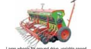
Large wheels for ground drive, variable speed gearboxes, plants small to large seeds, built in trays, fluted roller distributors, spring release covering harrows, row markers with hydraulic lift, 3pl floating lower link, walkway to access seed box. Available models: 3.0M 23 ROW
