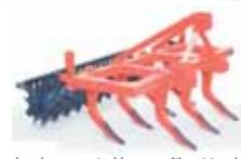
Break up hard compacted layers without turning soil over, correct tine submersion angle allows for maximum tractor output power. Crumble roller included.
