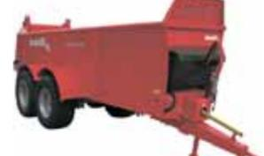
EVR 21-15, 20.04m<sup>3</sup> capacity, tandem axle model, incorporates, all Jeantil features and spreading technology.
