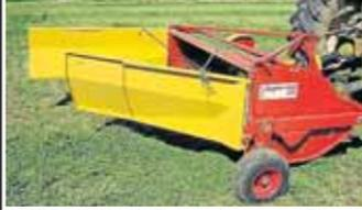
High speed hay & silage swath aerator conditioner. TED 160 includes standard wheels. TED220 includes castor wheel kit.
