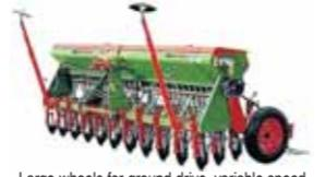
Large wheels for ground drive, variable speed gearboxes, plants small to large seeds, built in trays, fluted roller distributors, spring release covering harrows, row markers with hydraulic lift, 3pl floating lower link, walkway to access seed box. Available model: SLD20 & SLD24.
