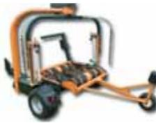
The high speed trailed model. Dual stretch dispenser (70% & 55%). Film break sensors. Hydraulic cut and start. Wide low ground pressure tyres and 6' easy load film roll holders.
