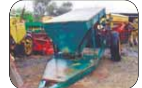
15 CWT 3/4 TONNE CRUMP MESSMATE Spreader (ground drive).
