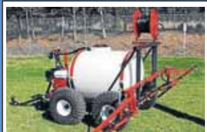
Trailer ATV 400 Litre. Twin axle hinged drawbar with damper. 8 metre boom with trapeze self leveler. Honda D/C to Bertolini 40 bar pump. Separate 3 section low pressure controller for boom with electric main ON/OFF. List price $7,653.00 incl. GST
