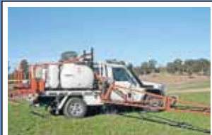
Tray mounted sprayer. 1200 Litre Pro Series. 12.5 Boom. Flush. Hydraulic boom lift and wing tilt both sides. Rate controller. Hydraulic assisted unloading. Electric start in cab. Foam or GPS can be fitted. (Super deal on Trimble 500) List price $34,196.00 incl. GST
