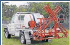
Pickup Sprayer 600 Litre with 6 metre boom attachment. Electric Main with separate low pressure controller for boom. Kohler 7 D/C to Bertolini 40 bar pump. High pressure reel 20m. Foam or GPS can be fitted. List Price $7,769.00 incl. GST.
