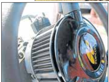
Topcon's electric steering wheel and GPS offer two centimetre accuracy without the expense and inconvenience of hydraulic installation. INSET: The electric steering wheel installed and ready for action.
