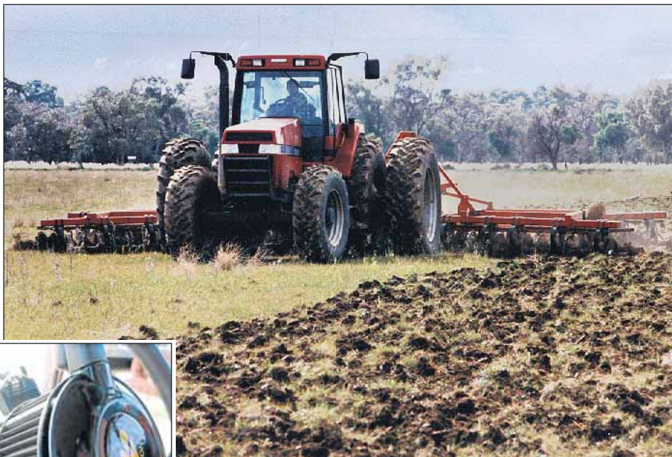
Topcon's electric steering wheel and GPS offer two centimetre accuracy without the expense and inconvenience of hydraulic installation. INSET: The electric steering wheel installed and ready for action.
