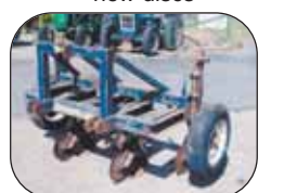
5 TYNE SUBSOIL PLOUGH with coulters 3pl (Colburn).
