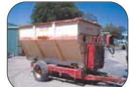
R.M.H. 4 ton mixer with elevator, PTO drive
